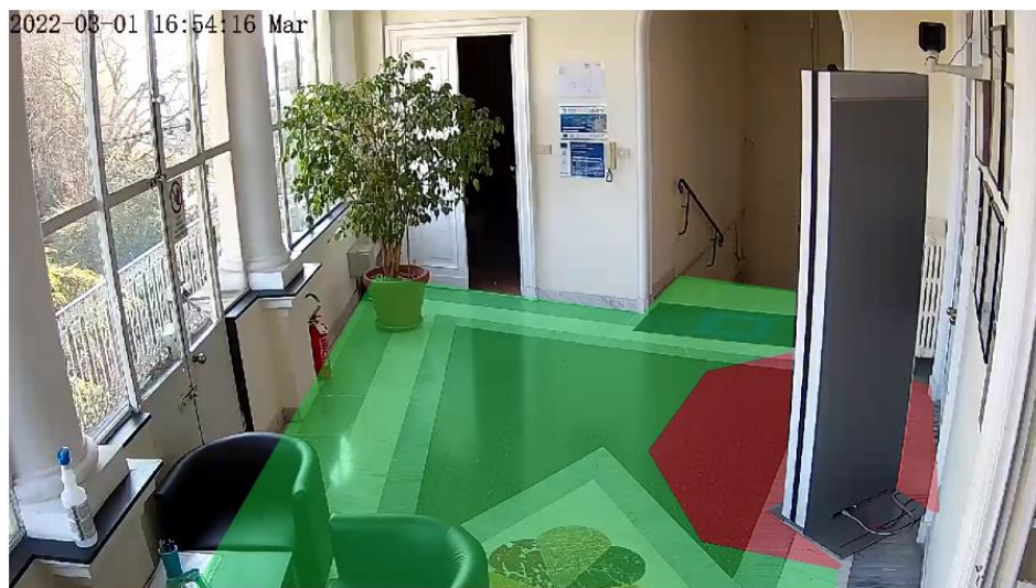
Figure 22 - Segmentation of a video frame acquired through a surveillance camera. Objects falling into these areas would trigger a proximity alarm.
