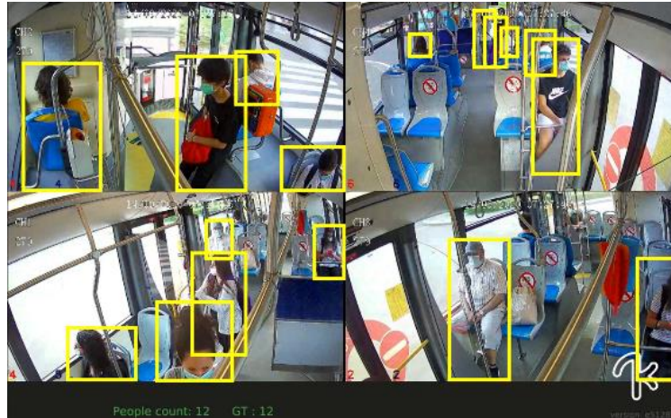
Figure 20 - Yolov4 output on a video frame.
