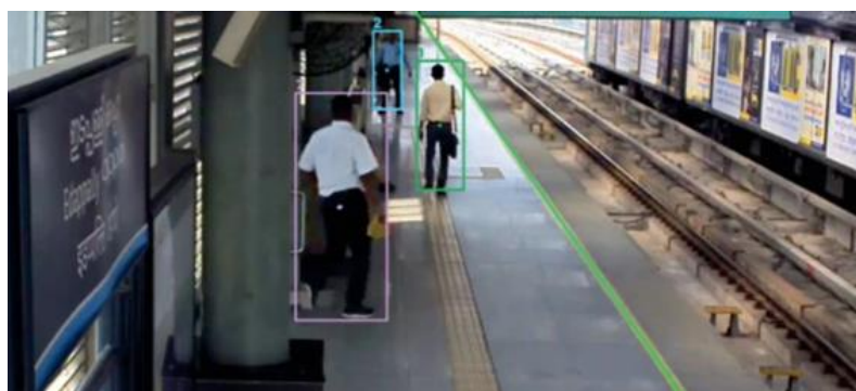
Figure 16 - Yolo detecting persons in the platform [9].
