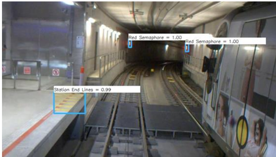
Figure 13 - Station End line detection with Yolo algorithm.
