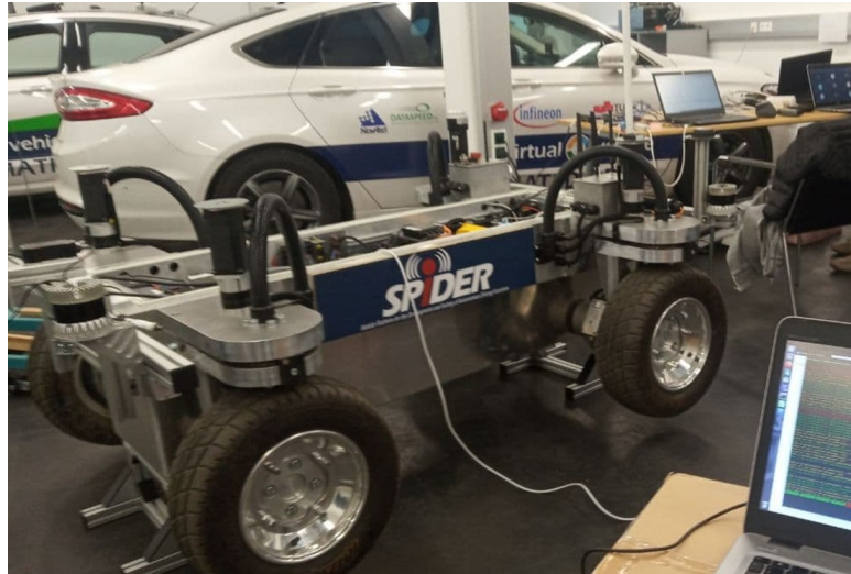
Figure 30 - SPIDER hardware tests, jacked up in garage
