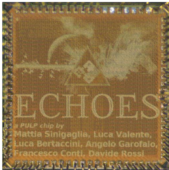
Figure 21 Echoes Chip - A Low-Power PULPissimo-based Chip
