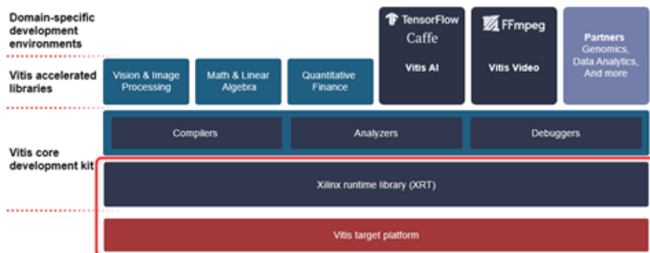
Figure 25 – Deample: Vitis Unified Software Platform
