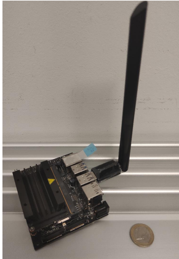
Figure 6 – Illustration of the test node equipped with TP-link AC1300 dongle
