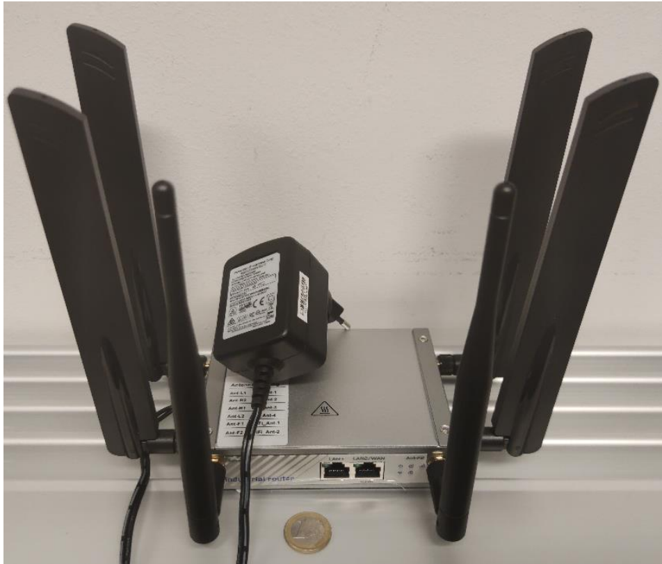
Figure 7 – Illustration of the TeleWell Industrial 5G AP used as IEEE 802.11 AP
