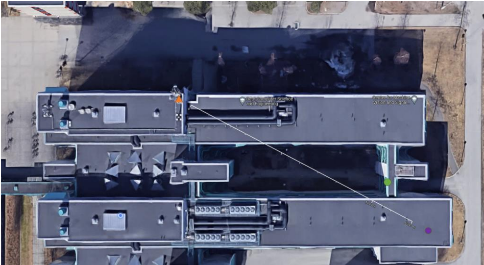
Figure 23 – Bird’s view on the experimental location (orange triangle denotes the position of 5G base station’s antenna, green circle marks the test location for tests ID 7-10, and purple circle signals the test location for tests 1-6.
