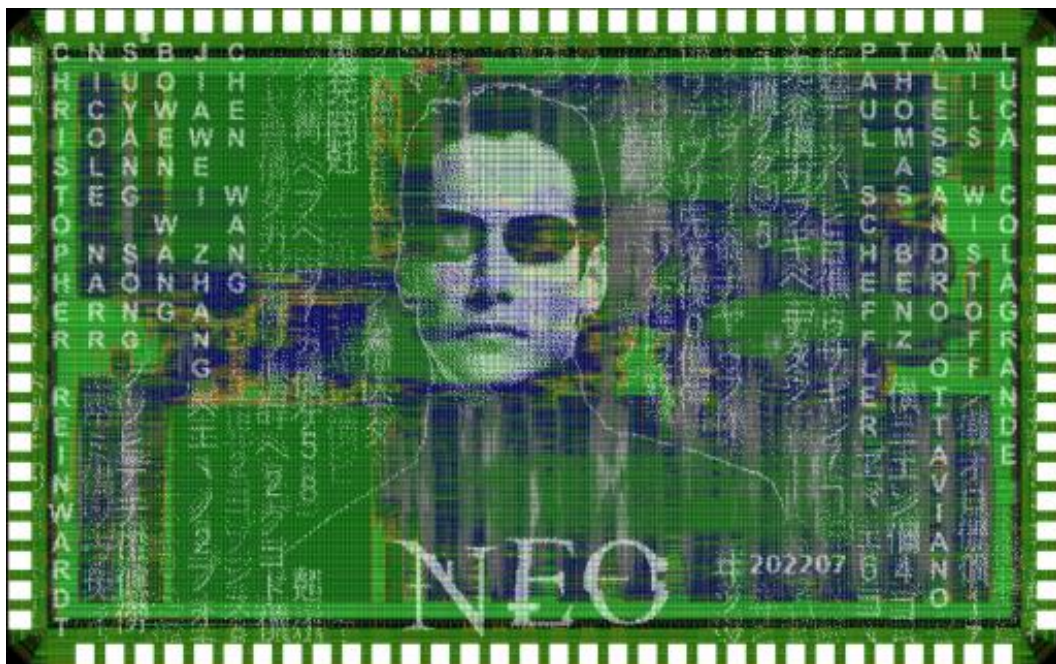
Figure 18 Neo, an Ariane/CVA6 implementation in TSMC65nm using the codebase supported by FRACTAL developments.
